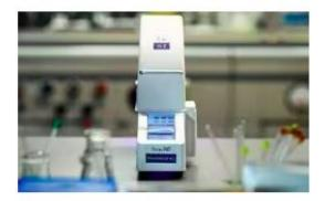
Photoreactors provide an all-in-one platform to consistently and reproducibly conduct photoredox catalyzed reactions. Each photochemical reactor consists of a light source and a cooling system to maintain stability of the reactants and products.
